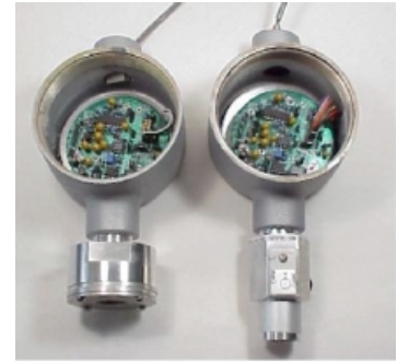
Figure 2: IST uses two types of electrochemical sensors: Type I (left) and Type II (right)
