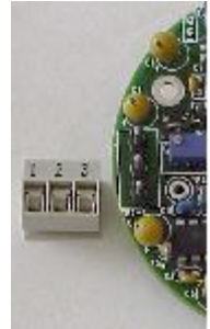
Figure 1 - The terminal block socket is provided within the transmitter
