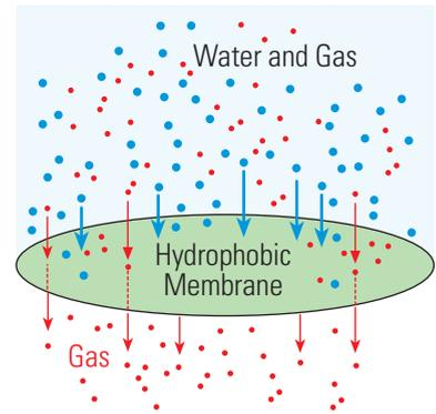
Fig. 4 Hydrophobic Membrane: prevents liquid electrolyte from leaking out.
