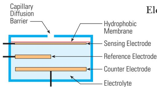
Fig. 3 Typical Electrochemical Sensor Setup
