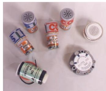
Fig. 1. Electrochemical Sensors
