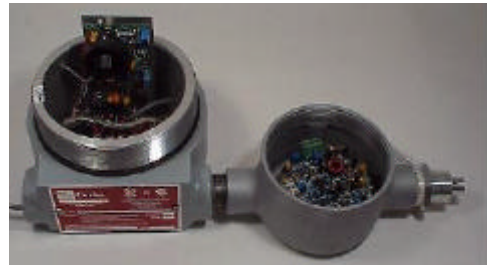
SM95-420I, isolated 4-20mA output for SM 95
